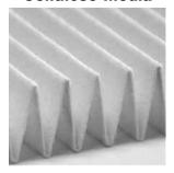
Traditional paper based media that provides a nominal level of depth filtration and capacity. Used with petroleum-based fluids only. Some grades of cellulose include a layered glass fiber substrate to provide more efficiency.
