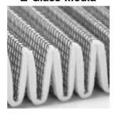
Multi-Layered, non-woven glass media that provides the highest levels of depth filtration efficiency and capacity. Higher capacity means longer service life. Coupled with a steel support mesh, Z-Glass can withstand higher differential pressures.
